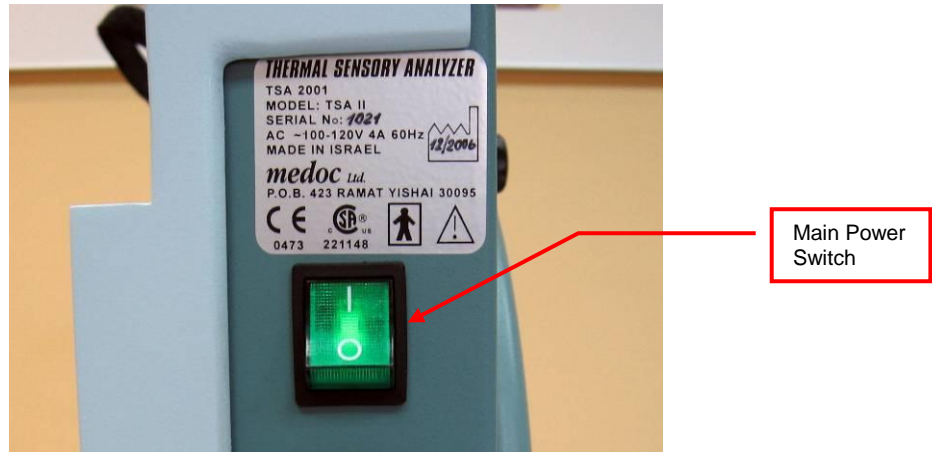
Figure 5: Main Power Switch
