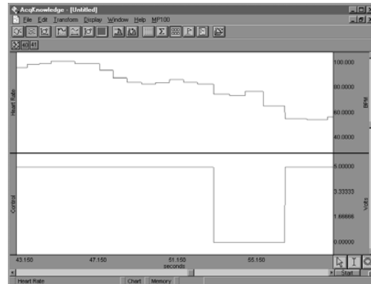
Control dialog and graph showing control channel switching from high to low when source channel is between 60 BPM and 80 BPM
