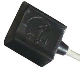
Tri-axial accelerometer uses 3 channel inputs
